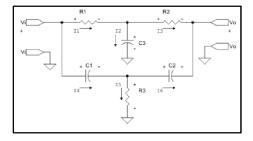
The twin T network is a rather unique RC network in that it can generated complex conjugates. Or in other words, you can get transfer functions that normally require inductors, without the use of inductors. This is why this network is used to make some rather special circuits. But first, we need to find out how this thing works. And despite the fact that this is a very simple little circuit, we are going to find that it is not quite so simple to
